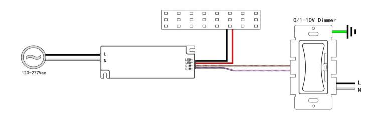
1. Input cable 2\*18AWG, Black cable to L, and White cable to N of Mains AC.
